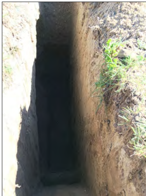
View looking at Pit 3 excavation. Note collapse of the left wall.
