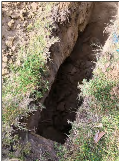
View looking at Pit 6 excavation. Note left wall collapse.
